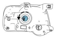
**WARNING:** Handle a halogen headlamp bulb carefully and keep out of children's reach. Grasp the bulb only by its plastic base and do not touch the glass. The oil from your hand could cause the bulb to break the next time the headlamps are operated.
